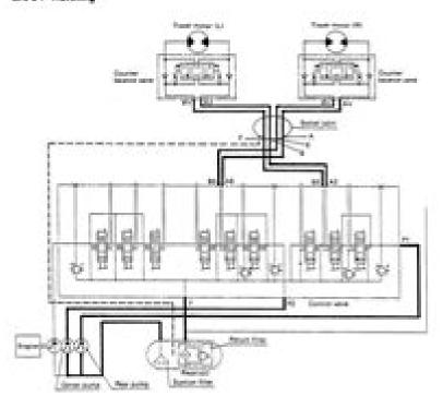
The main components of the travelling circuit include the hydraulic pump, control value, served part, counter-balance valve, based major with reduction
