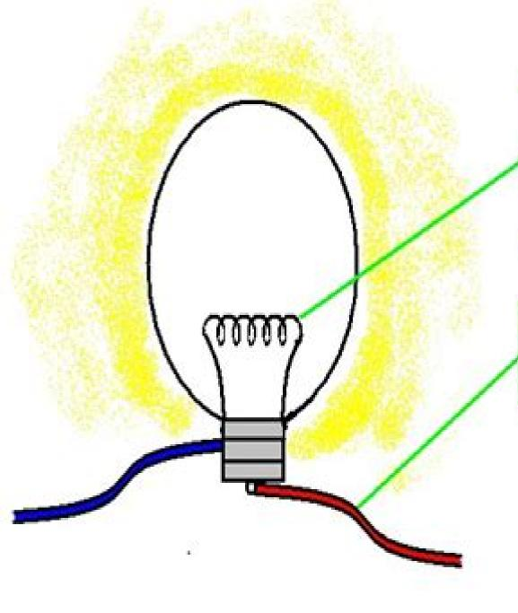
Resistance of light bulb filament is high to produces heat and light.
