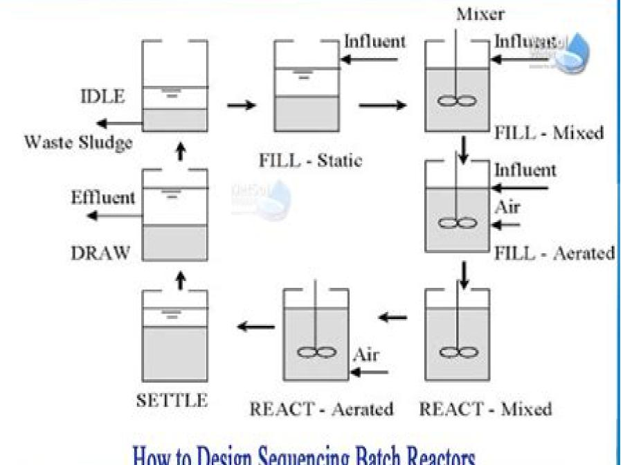
How to Design Sequencing Batch Reactors
