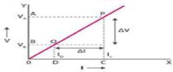
(b) Slope of V-I graph for a conductor represents resistance.
