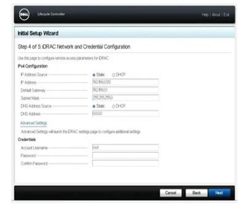
Figure 6. iDRAC Network and Credential Configuration page
