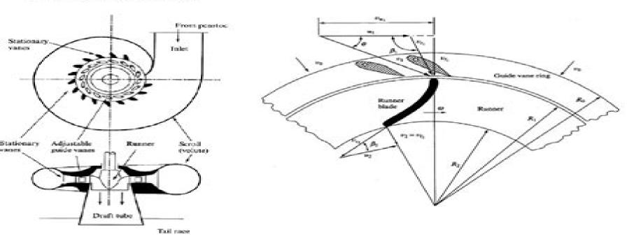
Figure 1 & 2- Schematic View and Velocity Diagram of Francis Turbine
