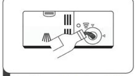
Carefully pour in the rinse-aid into its dispenser, whilst avoiding it to overflow.
