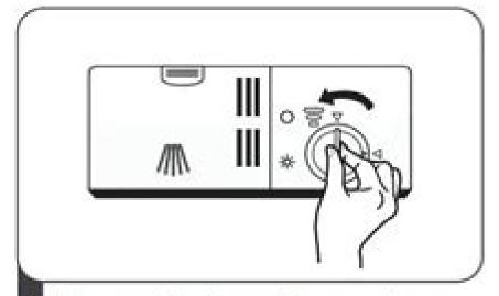
Remove the rinse aid reservoir cap by rotating it counterclockwise.
