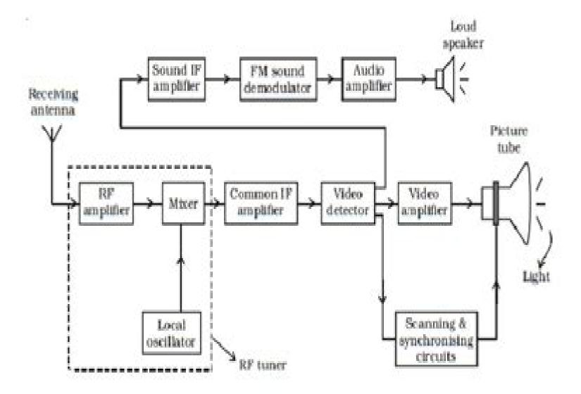
Elementary block diagram of a monochrome TV receiver
