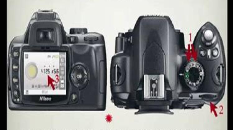
To choose a Shutter Speed, turn the mode dial and select Shutter Priority or Manual Mode, then adjust the command dial. Your Shutter Speed selection can be seen in the monitor.
