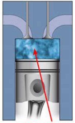
Low-Temperature Combustion: Ultra-Low Emissions (<1900K)
