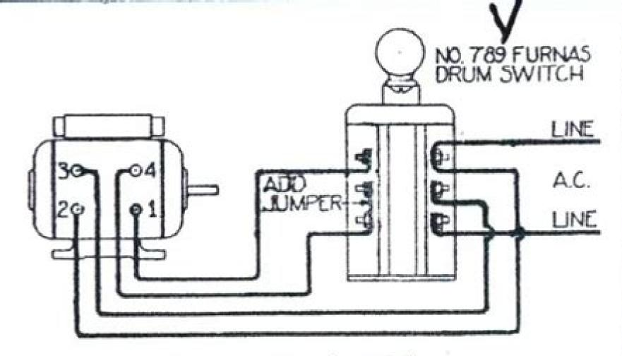
MOTOR-GEN ELEC. CAPACITOR (4-WIRE)
