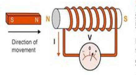
Faraday's Law of Electromagnetic Induction states that a changing magnetic field induces an electric current in a conductor.
