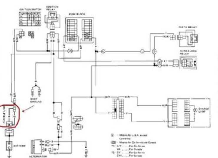
Fig. 239 Charging System Wiring Circuit
