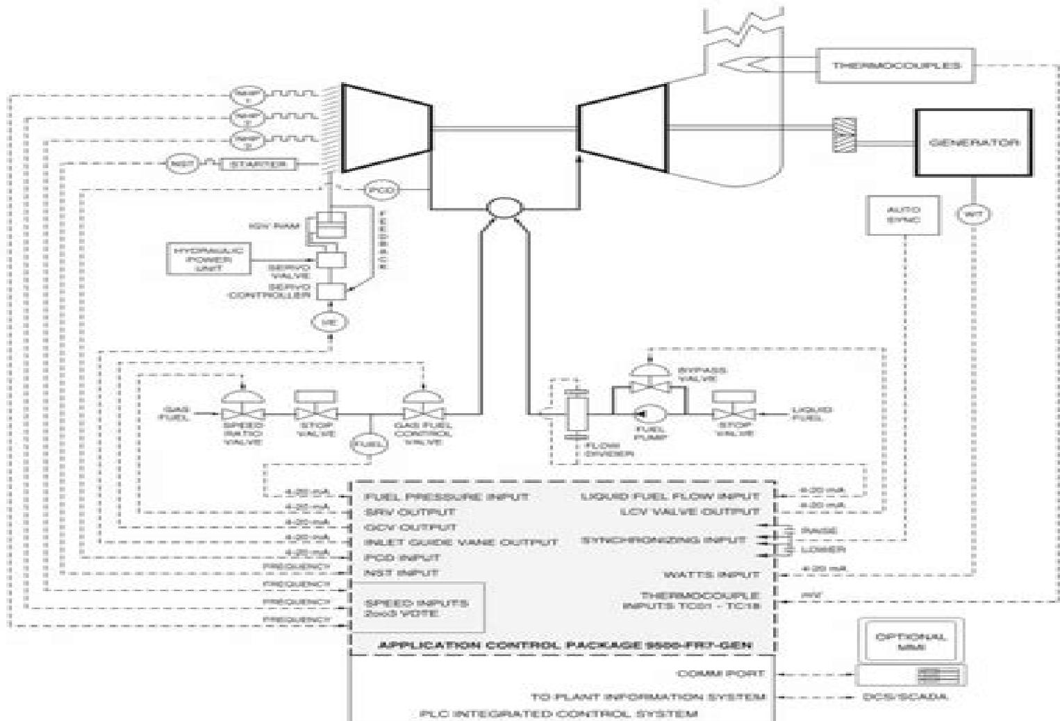
Simplified schematic showing a Petrotech GE Frame 7® gas turbine generator drive application control package integrated into an advanced PLC-based control system. Shown with dual fuel system.
