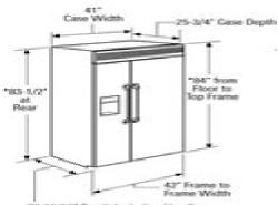
Shipping height. The refrigerator can be adjusted to fit into a cutout that is 83-1/2" min. to 84-1/2" max. height. Note that the top case trim at the front is 1/2" higher and will overlap upper cabinetry or soffit. Use leveling legs and wheels for a maximum 1" height adjustment.
