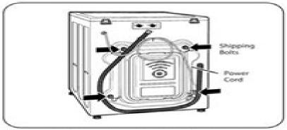
Starting with the bottom two shipping bolts, use the wrench (included) to fully loosen all four shipping bolts by turning them counterclockwise.
