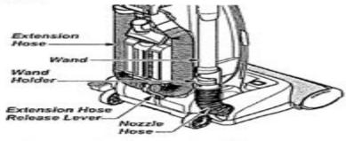
Remove the lower end of the extension hose from the wand holder by grasping the hose collar, twisting, and pulling straight up.
