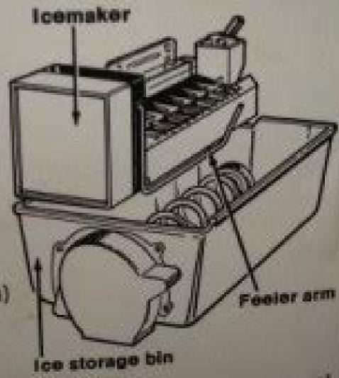
First cubes normally freeze after several hours. Discard all cubes from the first few batches (16 or 24 cubes) to flush impurities batches (16 or 24 cubes) to flush additional
