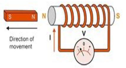
When the magnetic field around a conductor changes, it produces an electromotive force (EMF) that drives an electric current.
