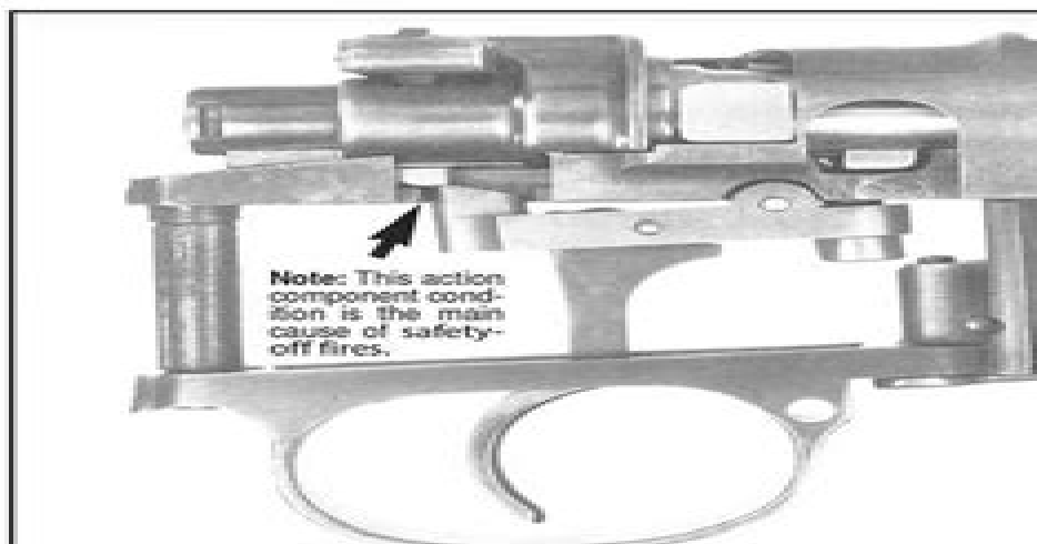
Figure 48- Shows the trigger sear in a cutaway M98 action blocked by cocking piece ledge overtravel that occurred when the trigger was cycled while the safety lever was in the safe position. This condition was caused by an altered top cocking piece safety lever engagement corner which reduced cocking piece/trigger clearance to less than zero. Note that this disconnects and blocks the trigger sear.
