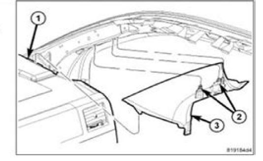
Using a trim stick C-4755 or equivalent, release the retainer clips (3) and remove the top cover.
