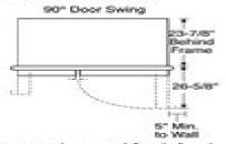
Allow minimum clearances for freezer door and fresh food door for a full 130° door swing and to allow for pan removal.
