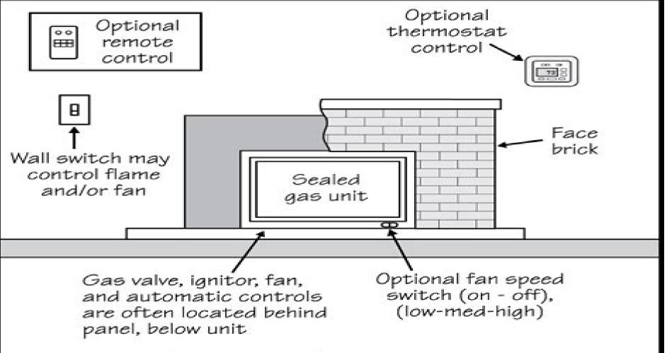
Sealed combustion gas fireplaces have various control options, including 110-volt switch, fan speed control, remote control, gas valve and/or thermostat control.
