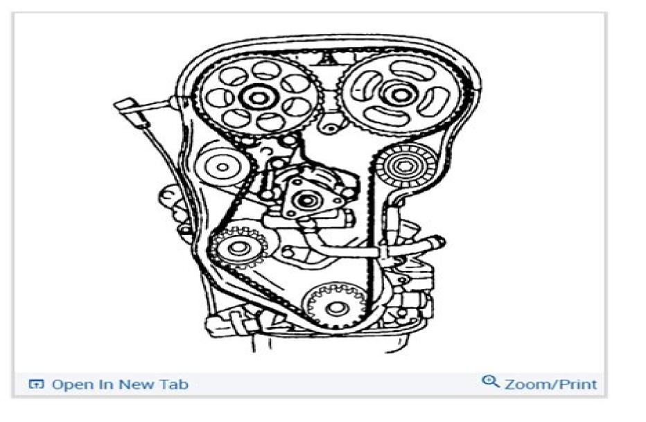
21. Important: Remove the timing belt behind the power steering pump.
