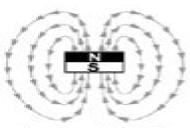
Any magnet will reach inside the magnetic field (the arrows)
