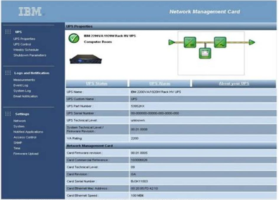
Figure 8. IBM LCD UPS Network Management Card (NMC) UPS properties window
