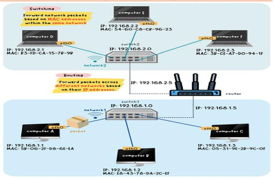
Gateway 📄 a "doorway" for traffic to flow in and out of the local network
