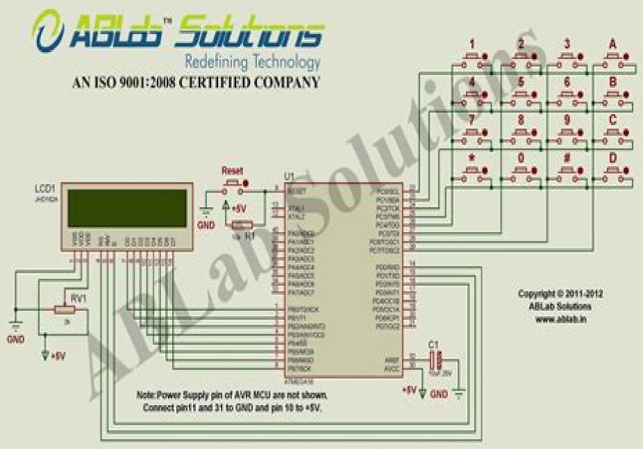
Circuit Diagram of 4x4 Keypad Interfacing with ATmega16 and LCD Display
