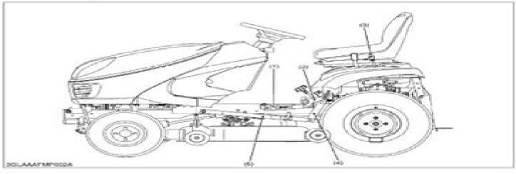
(1) Lift Cylinder (2) Lift Link Sheft (3) Hydraulic Lift Lever
