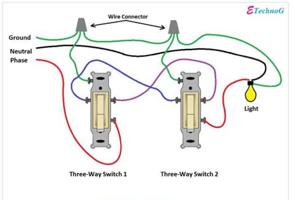
3 Way Switch Wiring
