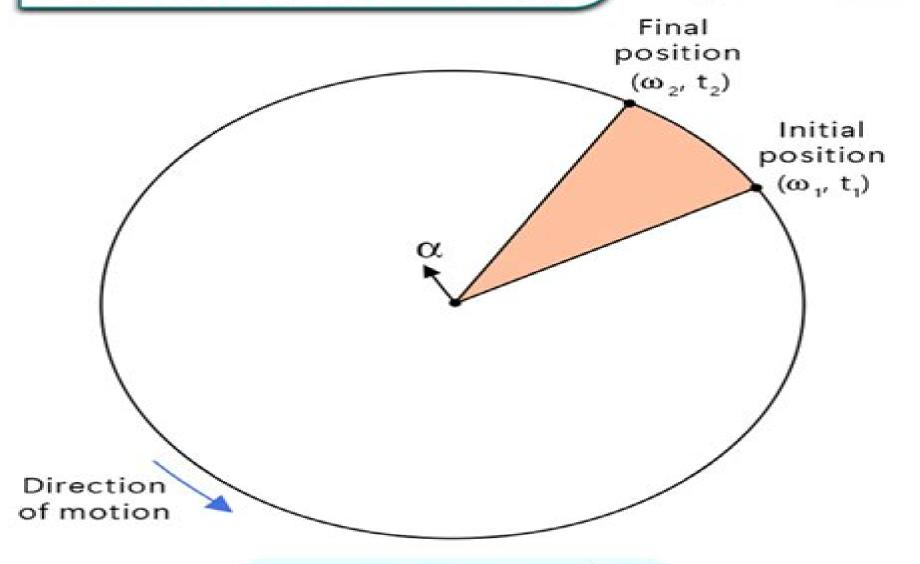
$$\alpha = \frac{\omega_2 - \omega_1}{t_2 - t_1} = \frac{\Delta \omega}{\Delta t}$$
