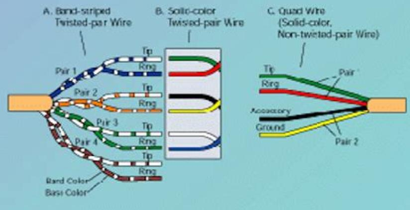
Note: For 6 wire jacks use pair 1,283 color codes. For 4-wire jacks, use pair 182 color codes.
