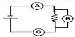
A) A is an ammeter and B and C are voltmeters. B) A is a voltmeter and B and C are ammeters.
