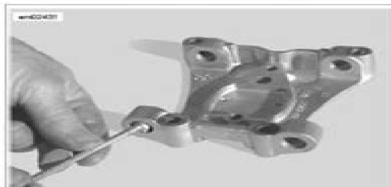
Figure 3-70. Checking Support Plate Bore
