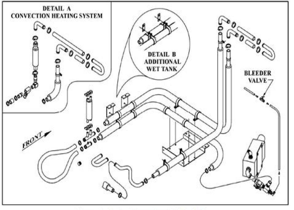
Figure 7—Engine Compartment Heater Piping
