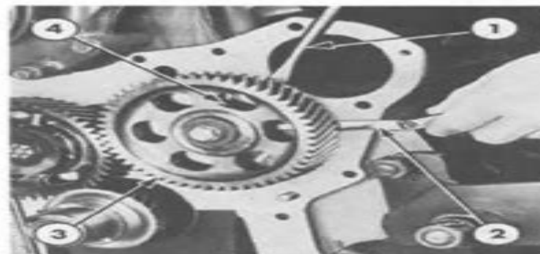
Figure 22 Measuring Camshaft End Play
