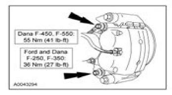
6. LAUTION: Never allow the rear disc brake caliper to hang from the brake hose. Provide suitable support.
