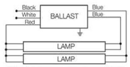
Note: For one lamp application, cap any blue lead. Insulate to 600 volts.
