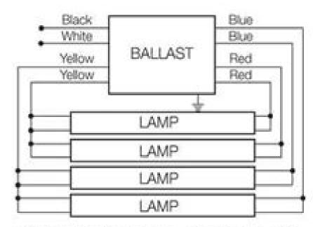
Note: For three lamp application, cap any unused blue lead. Insulate to 600 volts.
