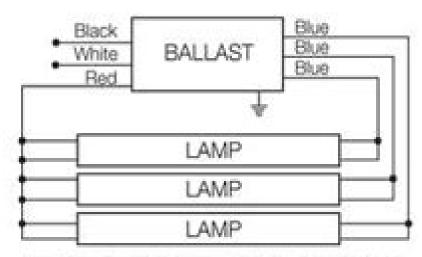
Note: For two lamp application, cap any blue lead. Insulate to 600 volts.
