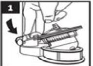
REMOVE OLD FLAPPER. MOUNT NEW FLAPPER.
