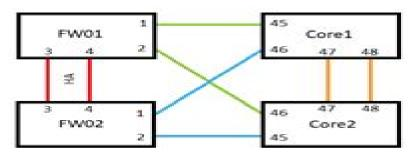
If 24 port core switches are used instead of 48, subtract 24 from the core port numbers
