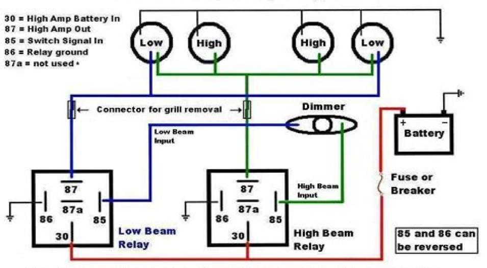
Headlamp harness should be upgraded to 14 ga wire throughout. OEM 1960 Chevy truck wiring shows 14 ga it green for high beams, 18 ga tan for low beams, 20 ga black grounds!
