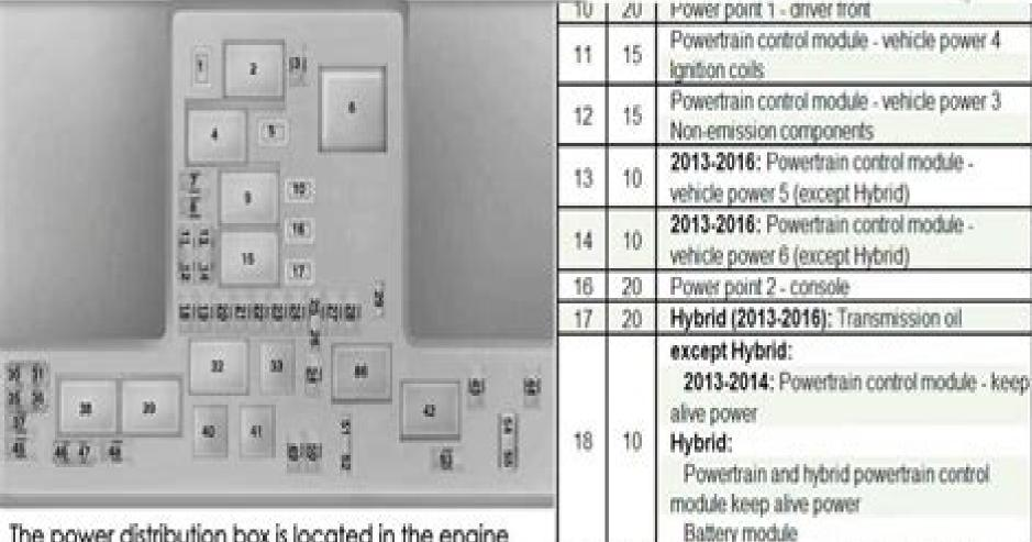
The power distribution box is located in the engine compartment. It has high-current fuses that protect your vehicle's main electrical systems from overloads.
