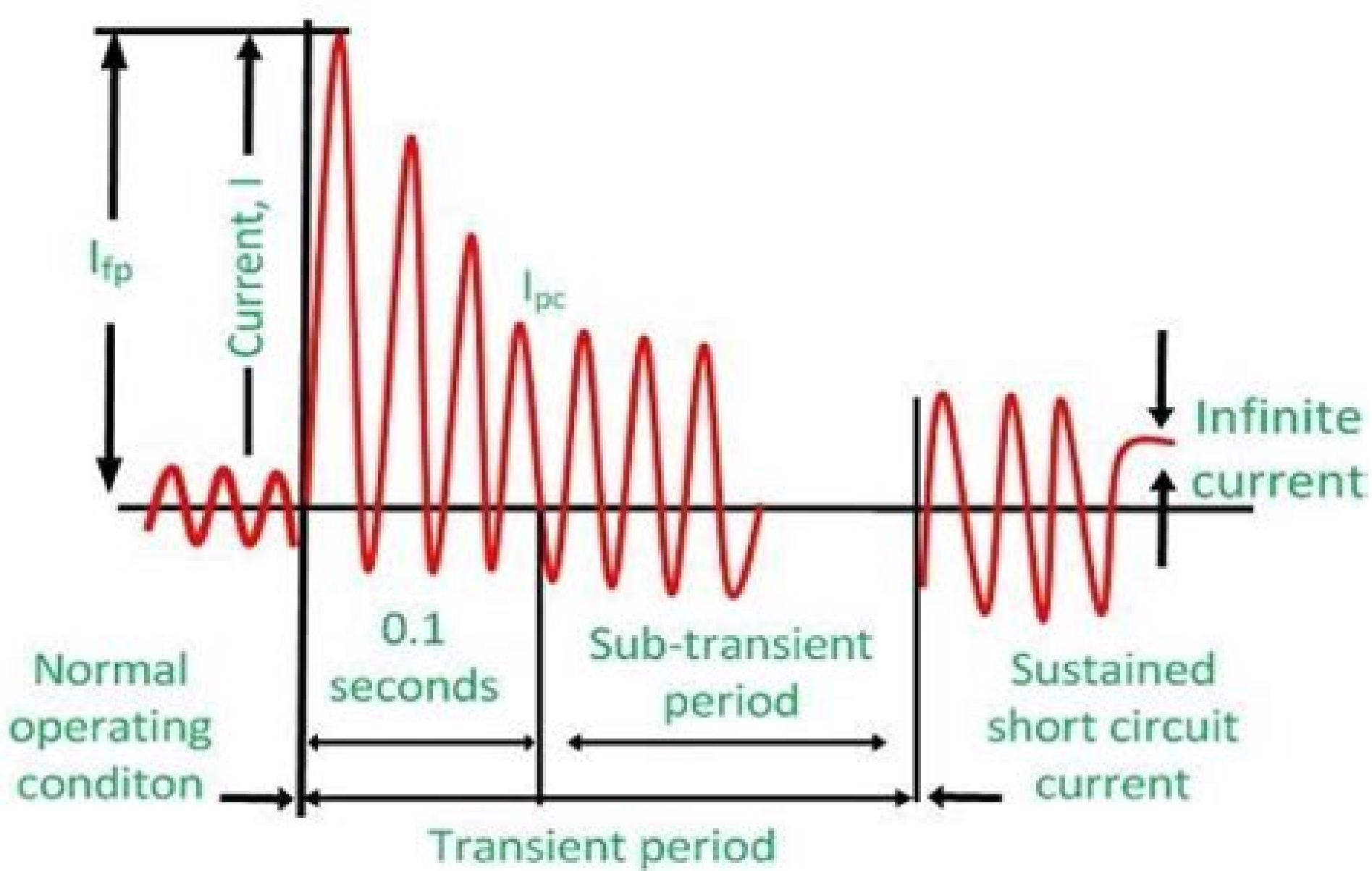
Process of Change in a Short-Circuit Current
