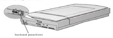
If the carriage does not automatically return to the home position, slowly raise the front of the scanner and hold it up until the carriage comes to rest in the home position. Then slide the transportation lock to the LOCK position.
