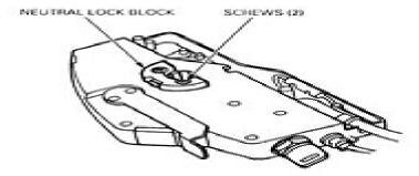
With the control lever in the neutral position, install it from the housing B side.
