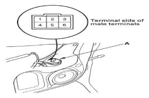
Test the motor in each direction by connecting battery power and ground according to the table.
