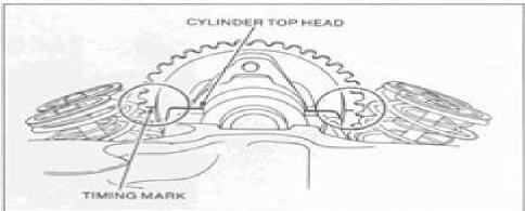
Slide the chain over the cam sprocket without rotating the sprocket.
