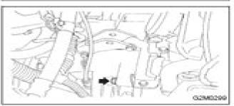
Remove bolt which holds right upper side of transmission to engine.
