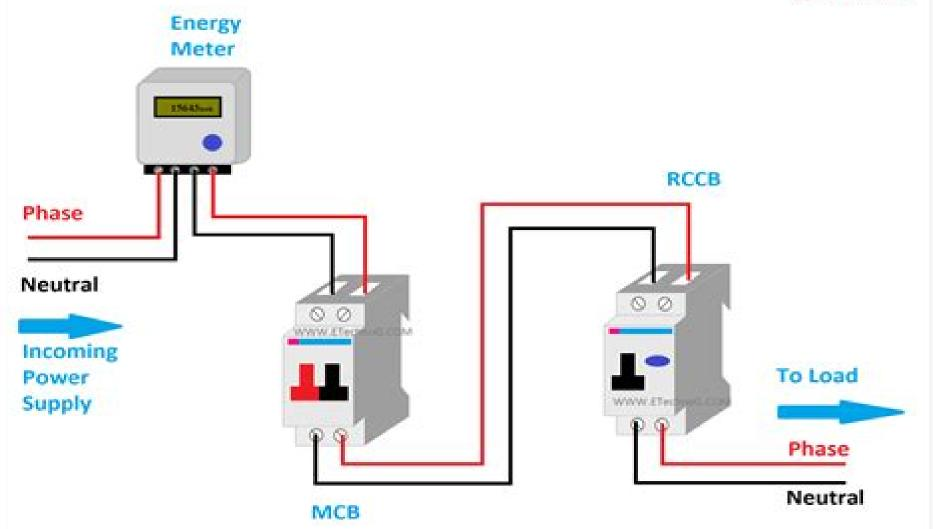
RCCB Connection Diagram with MCB
