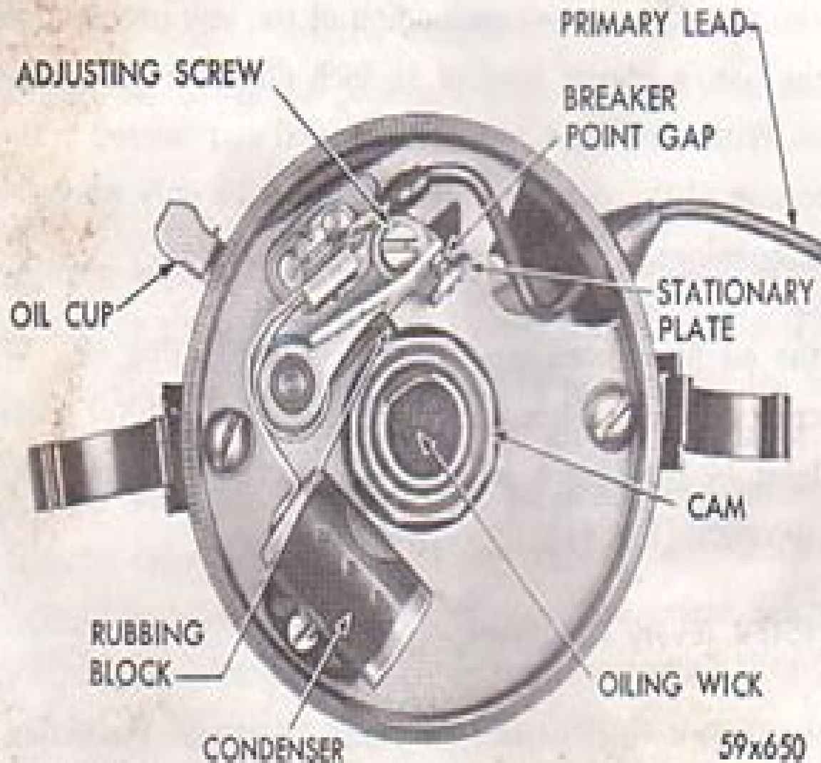
Figure 43—Distributor Lubrication Points
